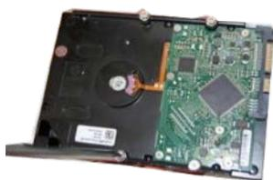
② Fix four screws in the HDD (Turn just three rounds).
