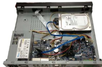
⑥ Connect the HDD cable and power cable.
