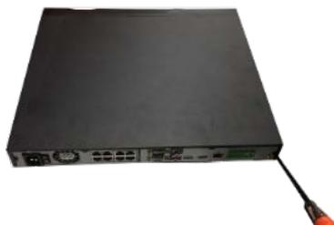
⑧ Secure the screws in the rear panel and the side
