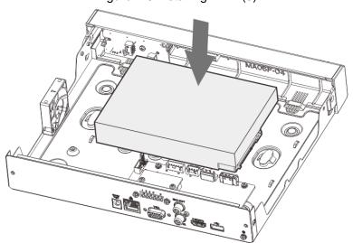
Step 4 Turn the device upside down, match the screws with the holes on the HDD and then fasten them. The HDD is fixed to the baseboard
