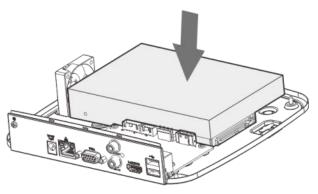
Step 4 Turn the device upside down, match the screws with the holes on the HDD and then fasten them. The HDD is fixed to the baseboard.
